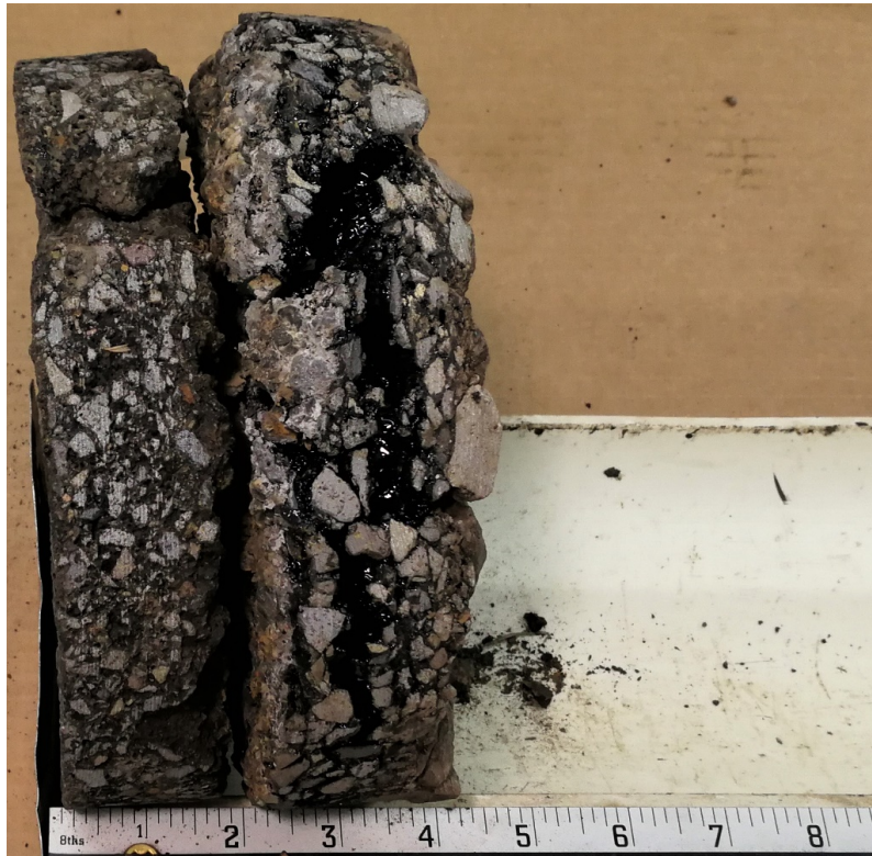
B-3 (Pavement Core Sample, 4.50 in.)
