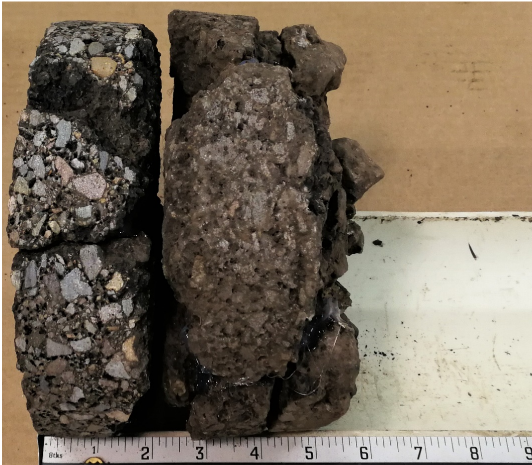
B-1 (Pavement Core Sample, 6.00 in.)
